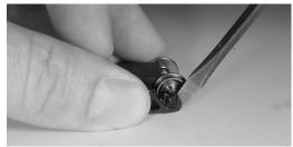
Use 1/8 inch Flat Blade Screw Driver and free axle on the opposite side that the wire exits the circuit box. **Important:** See next picture. Gently, pry each side frame out just far enough to free the axle from the side frame pocket.
