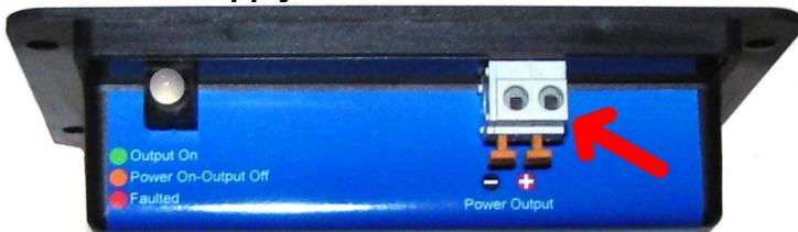
Connect the PWR-56 Track (+) and (-) terminals to each rail of the track. If you only have one PWR-56, it does not matter which track rail is connect to the (+) terminal and which track rail is connected to (-) terminal. Next plug the PA-2 Power adapter into the PWR-56 module. Finally, plug the power cable into the PA-2 and into a wall power outlet. The light should come on green. If it is not please see the PWR-56 troubleshooting table. See power supply section for complete details.
