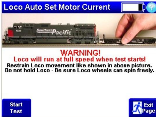
You will need to press the start button then restrain your locomotive like it shows in the picture above. In a few seconds, the auto feature will finish and display the measured motor full load current.
